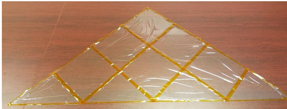
Figure 6.8: CP1 sail prototype with Kapton ripstops.
