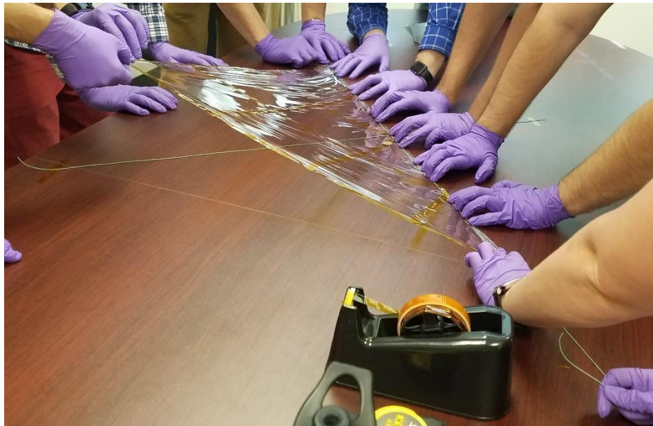
Figure 6.10: Folding process. Note the green Teflon wire used to define the folds.
