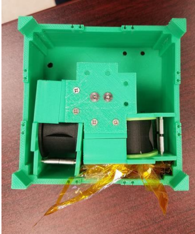
Figure 6.12: Fully folded CP1 sail quadrant in the allocated volume of a 3D printed prototype
