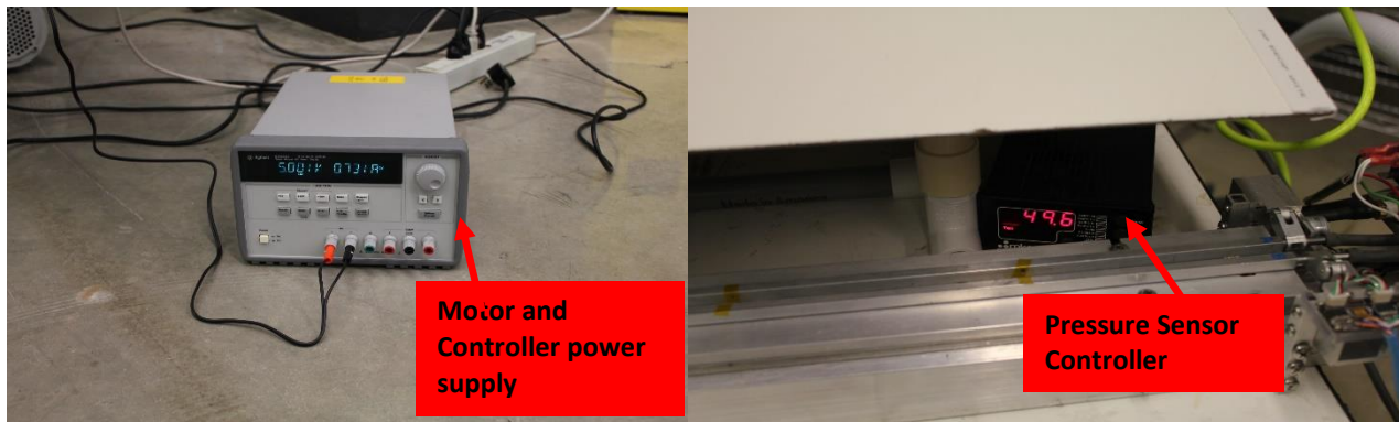
Figure 13.6: Power Supply and Pressure Sensor Controller
